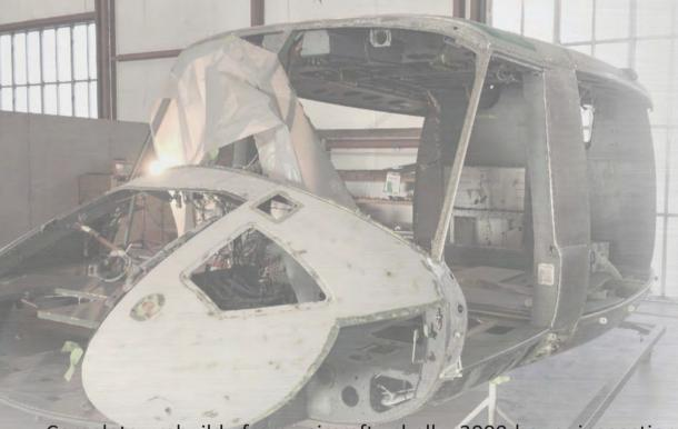
Complete rebuild from aircraft shell, 3000-hour inspection complete, cockpit upgrade, and NVIS installation.
